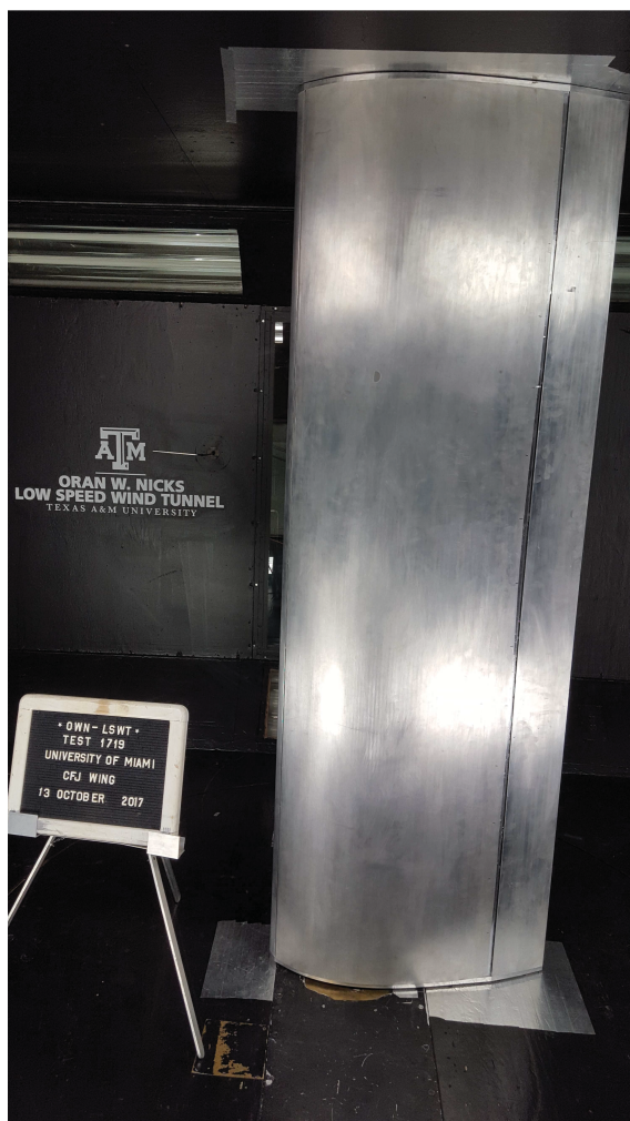
Figure 11.6: Photo of the CFJ-NACA-6421 airfoil tested.
