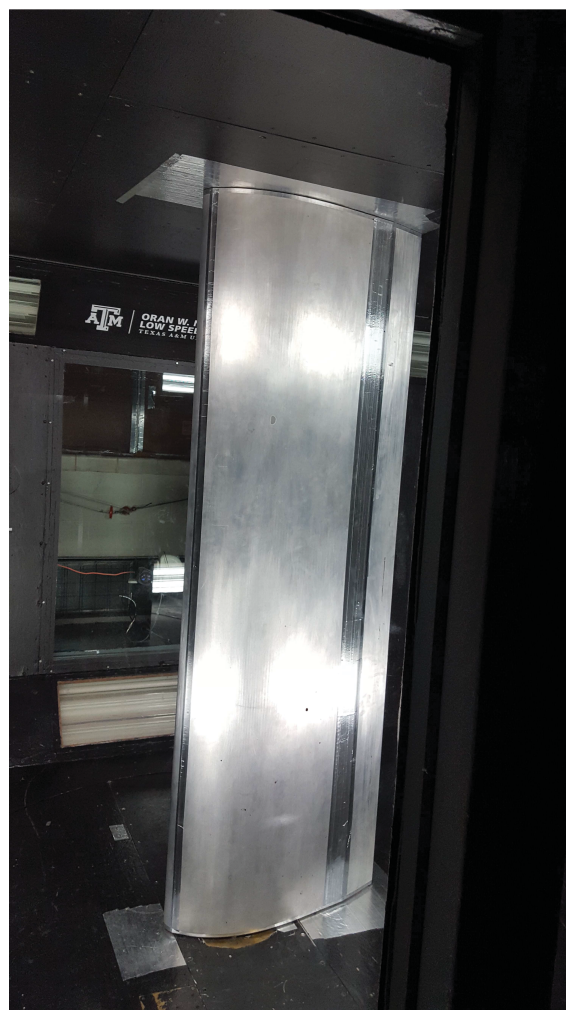
Figure 11.7: Photo of the baseline NACA 6421 airfoil tested.
