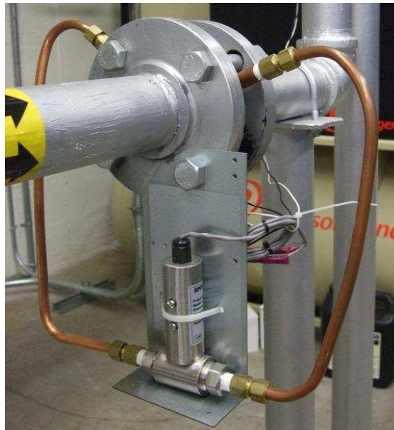
Figure 4.21: Spectre Sensors Model D150 Differential Pressure Transducer
