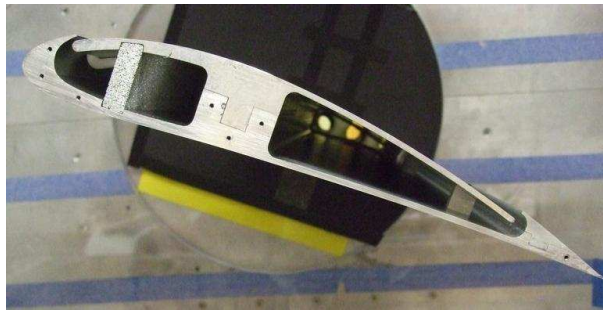
Figure 2.13: Cavities of Manufactured CFJ Airfoil
