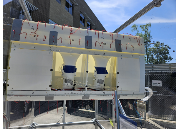
Figure 10: Inner structure of the micro-fan and ducts layout.
