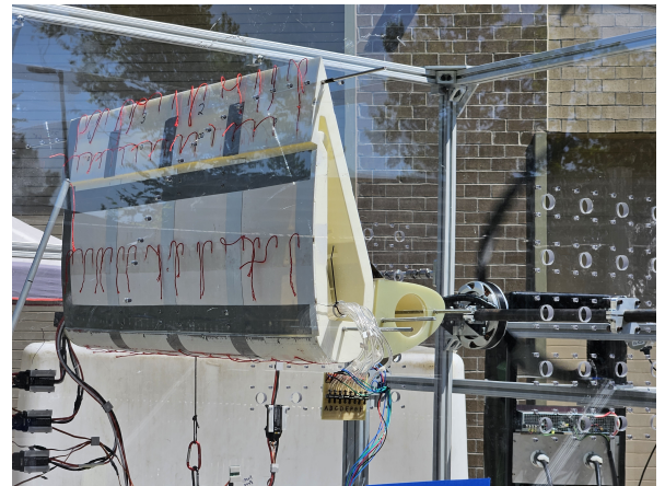
Figure 14: Tufts drop down when the jet is turned off.
