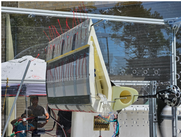
Figure 13: Tufts showing slipstream deflected 90^\circ by CFJ flap at 78^\circ during testing.
