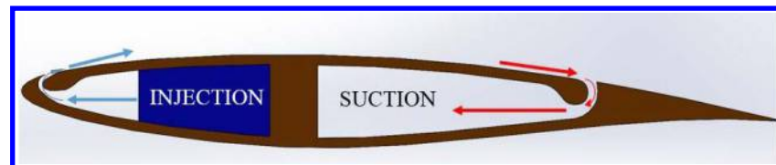
Fig 2. Cross section of airfoil along mid-span showing two cavities and slots
