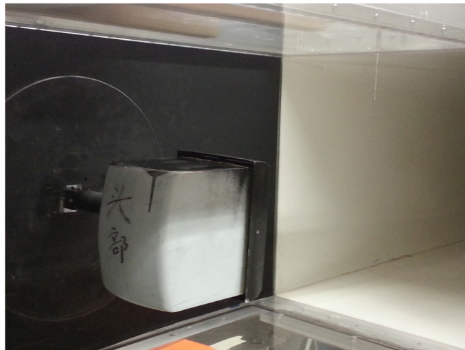
Figure 7b. The JBT bluff body installed in the wind tunnel for testing.
