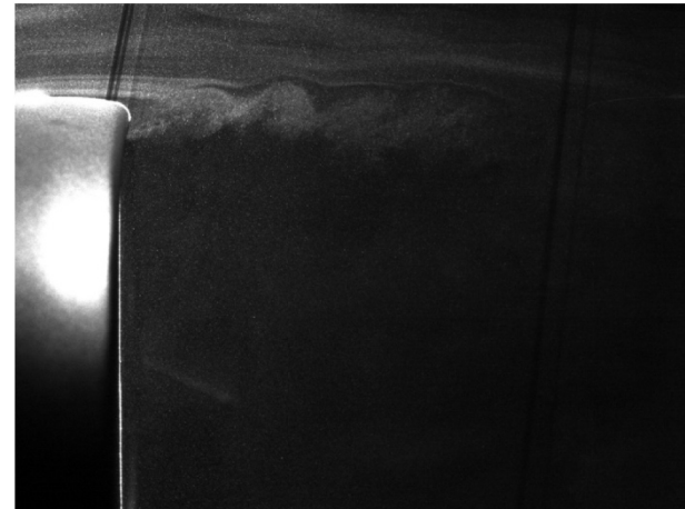
Fig. 12. Zoomed jet area of the jet mirror (tunnel 1) showing large coherent vortex structures.
