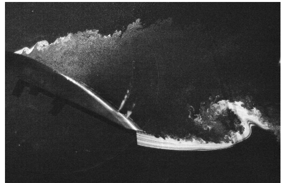
Figure 2.2: Massive flow separation of baseline NACA 6415 airfoil at AoA=25^\circ .
