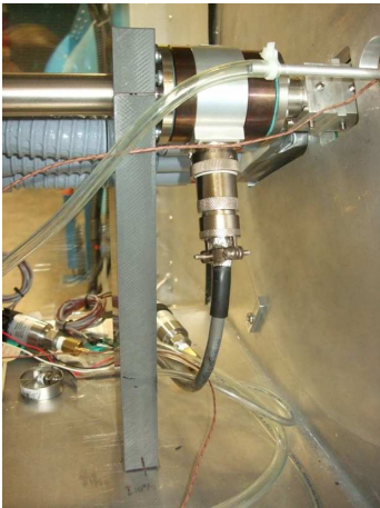
Figure 5.4: Sting support and force balance
