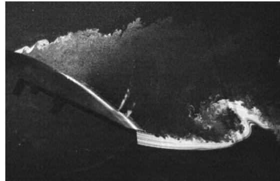
Figure 1.10: Implementation of CFJ on a generic airfoil.
