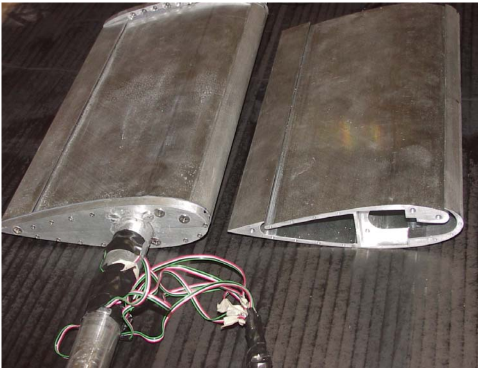
Figure 2-6. Connection between the balance cylinder and the airfoil
