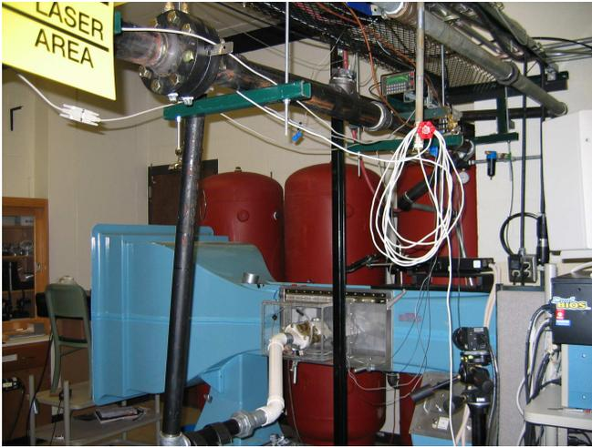
Figure 2: Wind tunnel setup and suction tanks.
