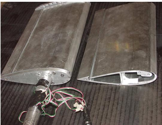
Figure 3: CFJ airfoil showing the injection side.
