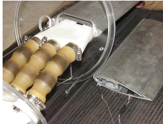
Figure 4: CFJ airfoil showing the suction side.
