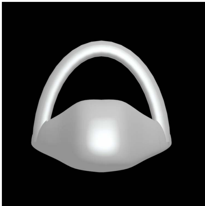
Figure 4. Front view of the PAV showing the wing dihedral angle of 5^\circ
