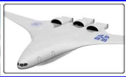
Figure 5: The concept aircraft SAX-40
