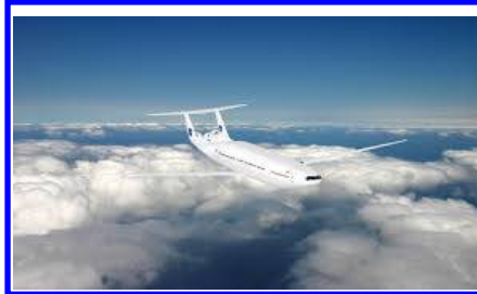
Figure 4: The Double-Bubble future aircraft concept by MIT
