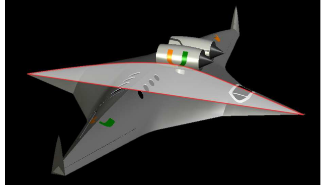
Figure 4: A SBiDir-FW civil transport in subsonic mode flying toward right, subsonic thick airfoil highlighted in the middle.
