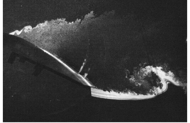
Figure 2: Massive flow separation of baseline NACA 6415 airfoil at AoA=25^\circ .
