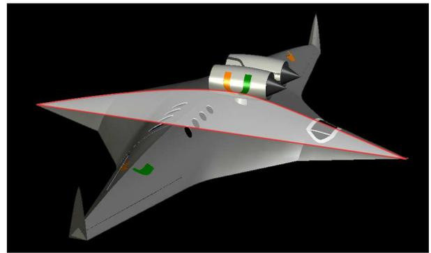
Figure 4: A SBiDir-FW civil transport in subsonic mode flying toward right, subsonic thick airfoil highlighted in the middle.
