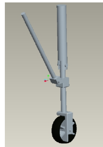
Figure 11: Landing Gear CAD Model
