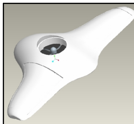
Figure 2. The MIRAGE's flying wing configuration in landing/take-off mode.
