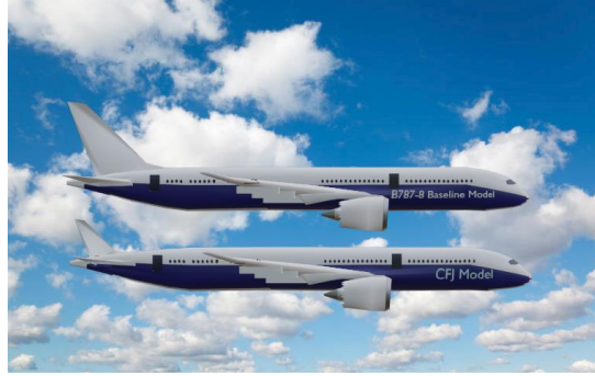
Fig. 8 B-787-8 Baseline and CFJ Model Comparison with 50% Empennage Reduction
