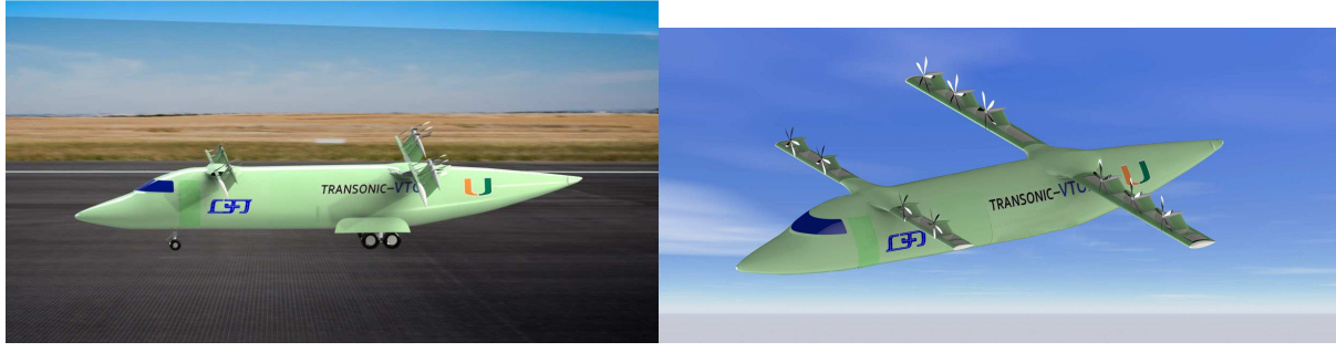
Figure 5. High speed CFJ VTOL from takeoff to cruise
