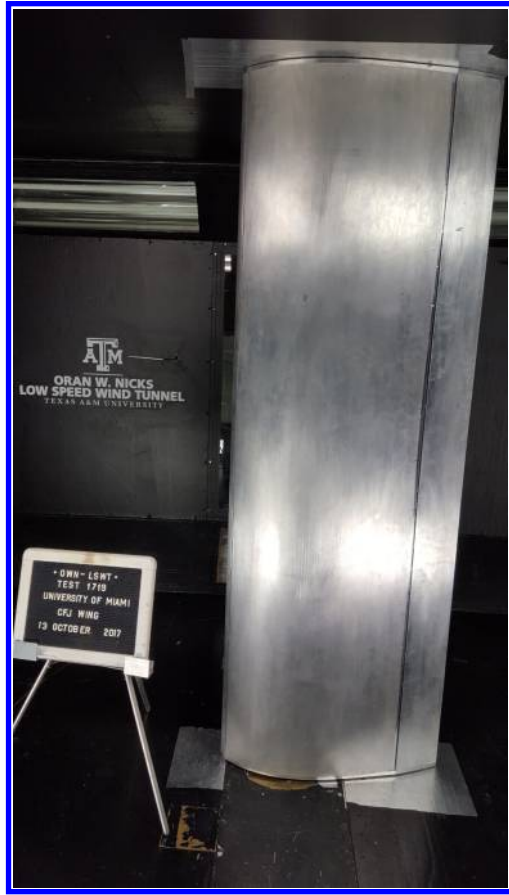
Figure 3: Photo of the CFJ-NACA-6421 airfoil tested.
