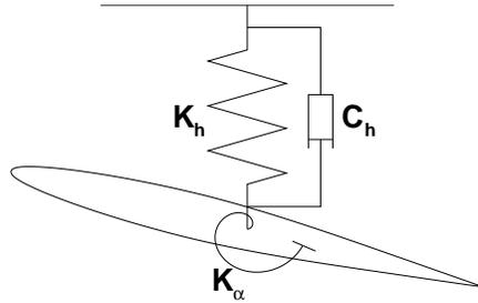
Figure 14: Sketch of the elastically mounted airfoil
