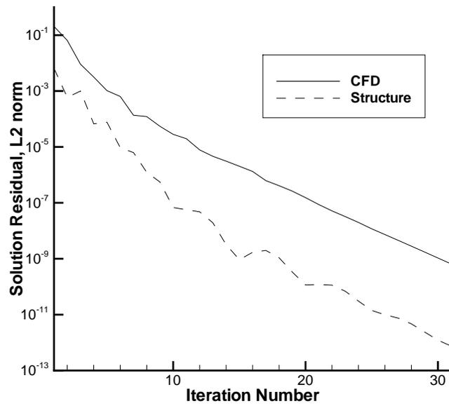
Figure 10: Convergence histories for both CFD and structural solvers within one physical time step
