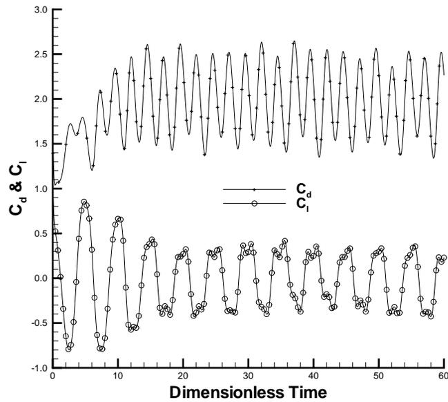
Figure 7: Time histories of the lift and drag coefficients of the oscillating cylinder,  $\mu_s = 5$ ,  $\zeta = 0.0403$
