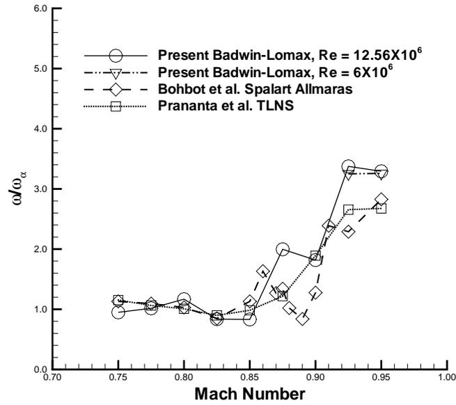
Figure 20: Comparison of computed flutter boundaries -  $\frac{\alpha}{\omega_\alpha}$  versus Mach number.
