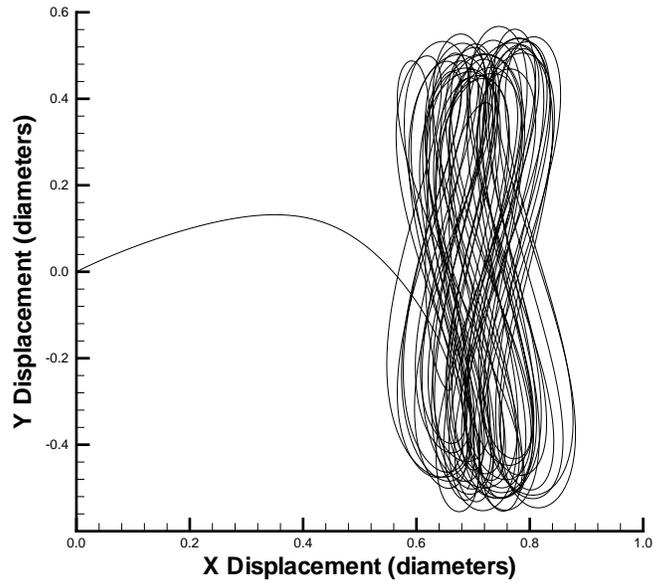
Figure 8: The trajectory of the Time histories of the lift and drag coefficients of the oscillating cylinder,  $\mu_s = 1.2732$ ,  $\zeta = 0.1583$
