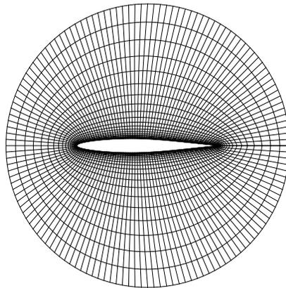
Figure 15: O-type mesh around the NACA 64A010 airfoil
