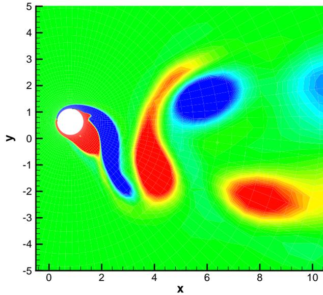
Figure 6: Vorticity contours with large cylinder structural oscillation amplitude,  $\mu_s = 1.2732$ ,  $\zeta = 0.01583$
