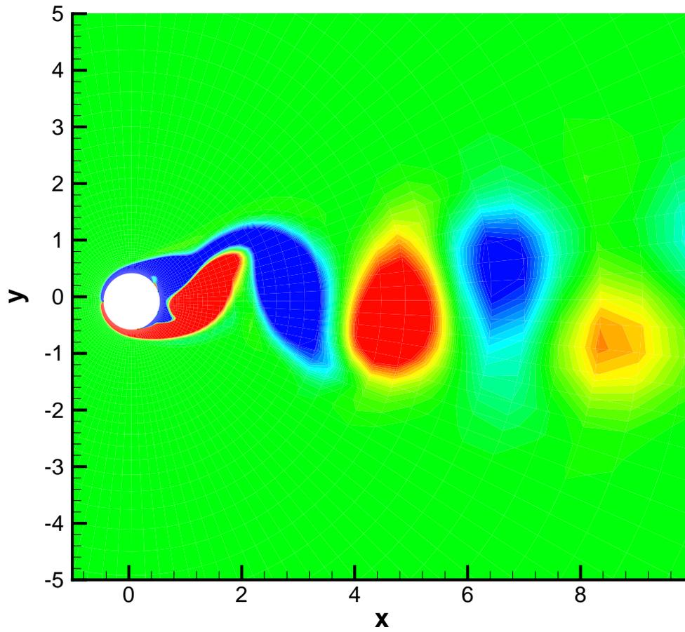
Figure 5: Vorticity contours with small cylinder structural oscillation amplitude,  $\mu_s = 12.7324$ ,  $\zeta = 0.1583$ ,
