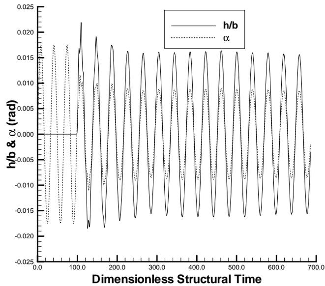
Figure 17: Time histories of plunging and pitching displacements for  $M_\infty = 0.825$  and  $V^* = 0.59$  - Neutrally stable response.
