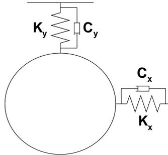
Figure 2: Sketch of the elastically mounted cylinder
