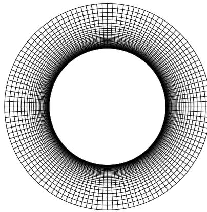
Figure 3: Mesh around the cylinder near the solid surface
