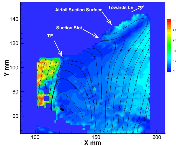
PIV of CFJ airfoil,  $\text{AoA}=46^\circ$ ,
