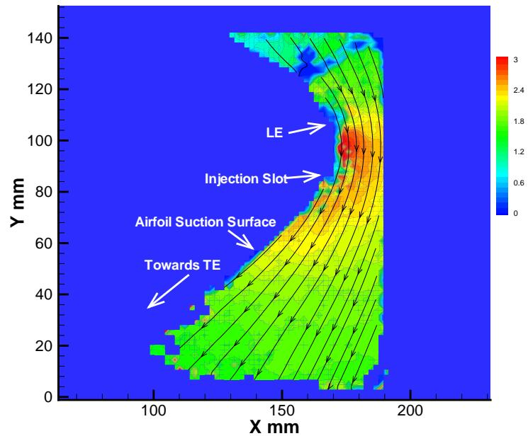
PIV of CFJ airfoil,  $\text{AoA}=43^\circ$ ,
