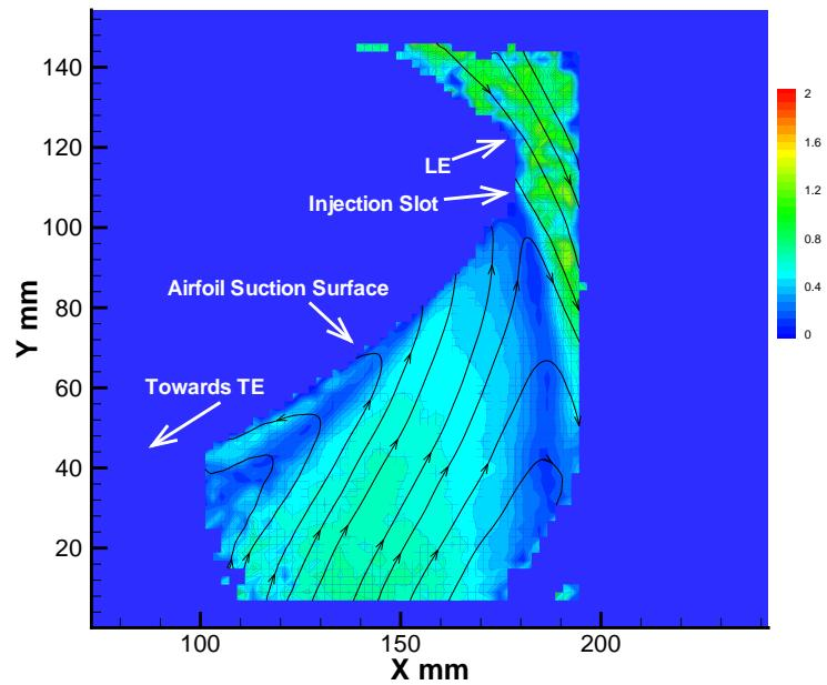
PIV of CFJ airfoil,  $\text{AoA}=46^\circ$ ,
