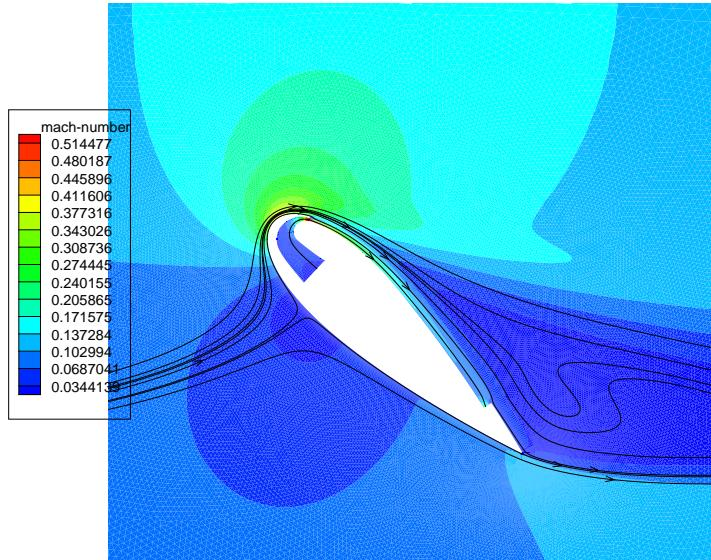
Computed CFJ airfoil Mach contours with streamlines at
