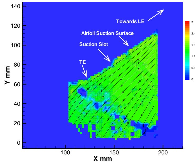
PIV of CFJ airfoil,  $\text{AoA}=43^\circ$ ,
