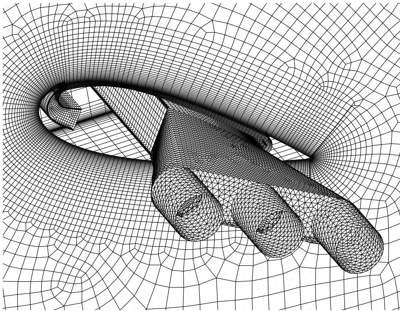
3D mesh of the CFJ airfoil inside the wind tunnel with secondary
